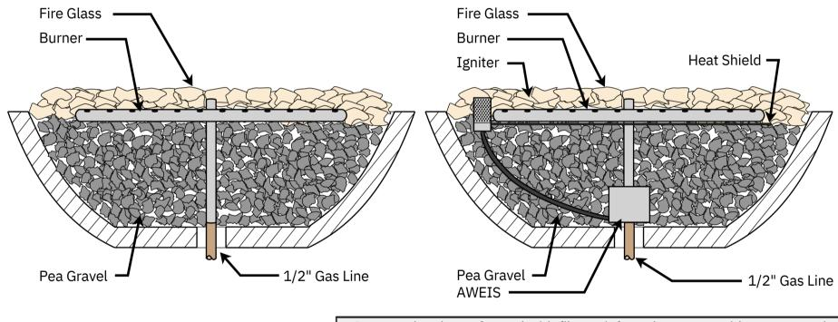
Concrete bowls are formed with fiber reinforced concrete with a water sealer additive and color all through the bowl. Cured for strength and durability.
