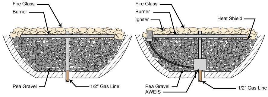
Concrete bowls are formed with fiber reinforced concrete with a water sealer additive and color all through the bowl. Cured for strength and durability.
