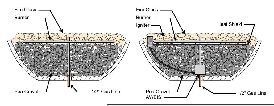
Concrete bowls are formed with fiber reinforced concrete with a water sealer additive and color all through the bowl. Cured for strength and durability. **Concrete Fire Bowl**
